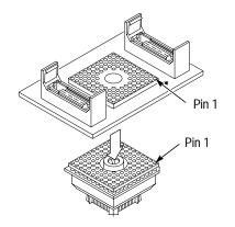
Figure 1–1: Connecting the test clip to the probe adapter
