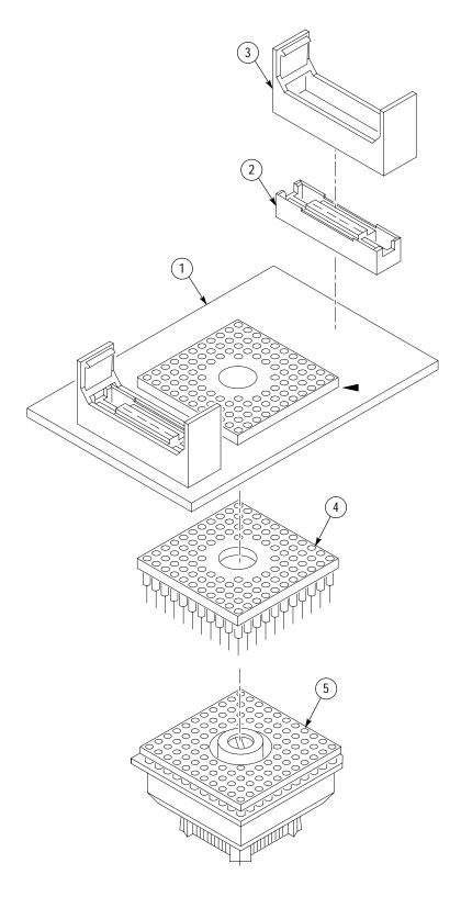
Figure 1: MCF5202/03 probe adapter exploded view
