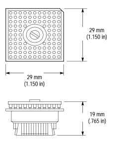
Figure 3-2: Dimensions of the test clip
