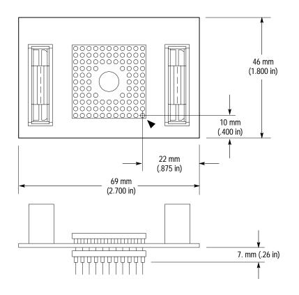
Figure 3–1: Dimensions of the probe adapter
