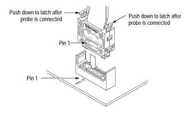
Figure 1–2: Connecting P6434 probes to the probe adapter
