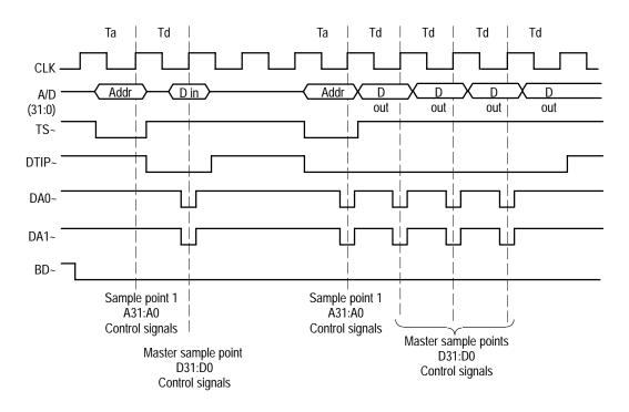
Figure 2–1: MCF5202/03 bus timing
